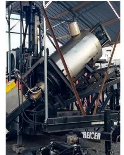
The inclined rotary gasifier developed at SCU (source: SCU).
